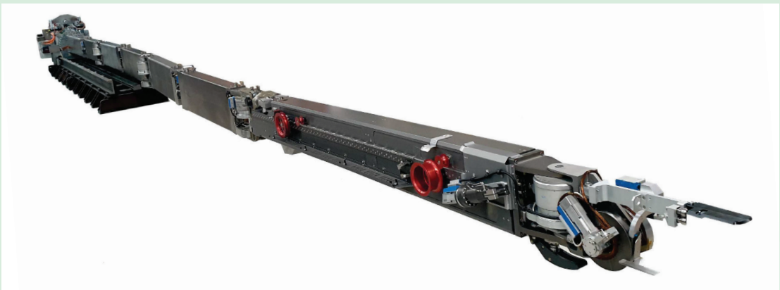
Left: VNS robotic arm for Fukushima investigation
