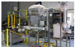
GeoMelt ICV Equipment Used for Demonstration Melts
