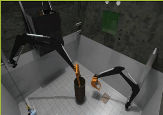
Remote Excavators for Hot Cell Clean-up
