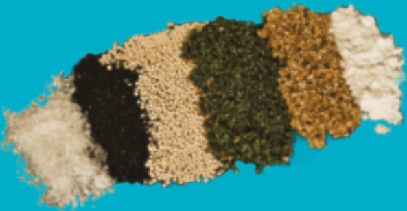
ISM are proprietary inorganic media used to remove undesirable ions from aqueous waste streams
